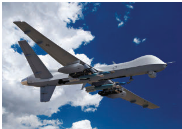
This artist's rendering of a future Predator B ER (Enhanced Endurance) UAV shows a potential version with fuel pods.
