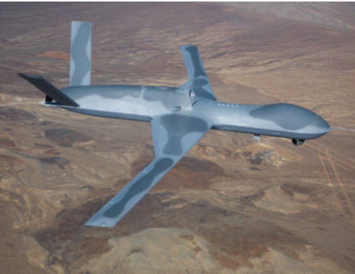
The General Atomics Predator C Avenger unmanned combat aerial vehicle, shown above, is jet powered, and is a candidate for the U.S. Navy's planned fleet of carrier-based fighting UAVs.
